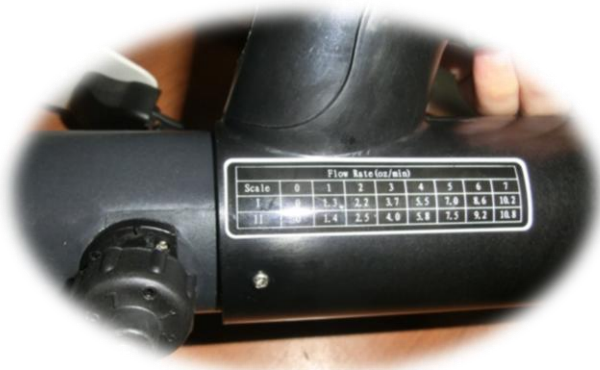
Adjustable orifices size for controllable flow rate
