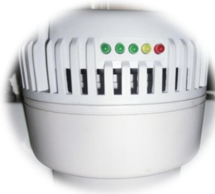
Indicative LED of battery level
